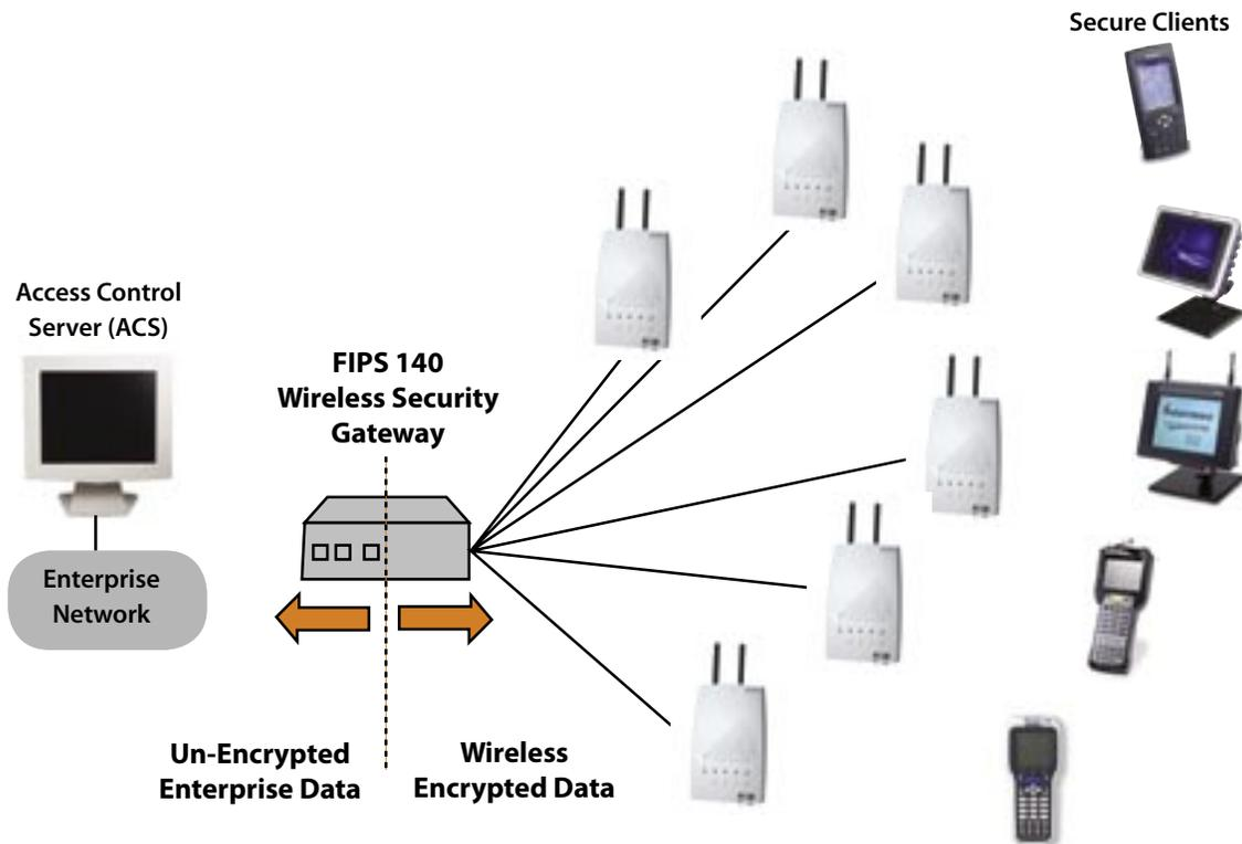
FIPS 140 provides data payload security (encryption), but not network security without firewall isolation and use of a VPN. FIPS 140 allows a number of encryption methodologies to be employed such as Advanced Encryption Standard (AES) or Triple Des (3Des). Some experts say that 3Des could not be broken by a supercomputer in 1,000 years. This is a much different data security approach than WEP and does not require key rotation.
